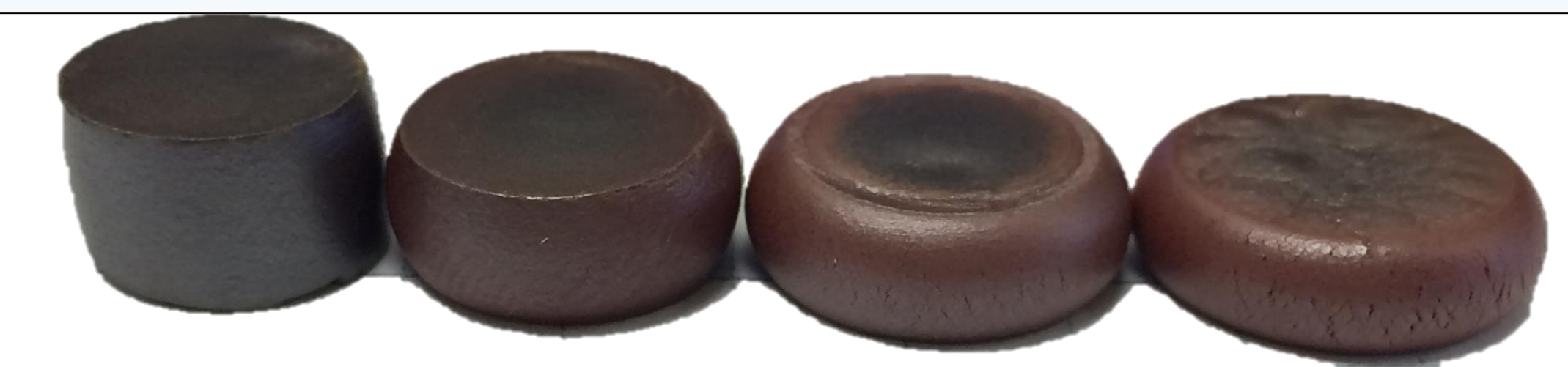
FIG 5: BiCuVOx forge samples (without templates) with increasing load, (l to r) 736, 1104, 1472, & 1839N
